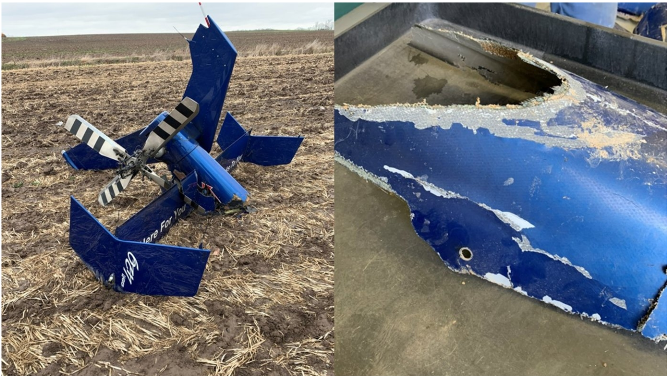
Figure 1 Figure 1 Tail rotor and main rotor blade slice in tail boom.
